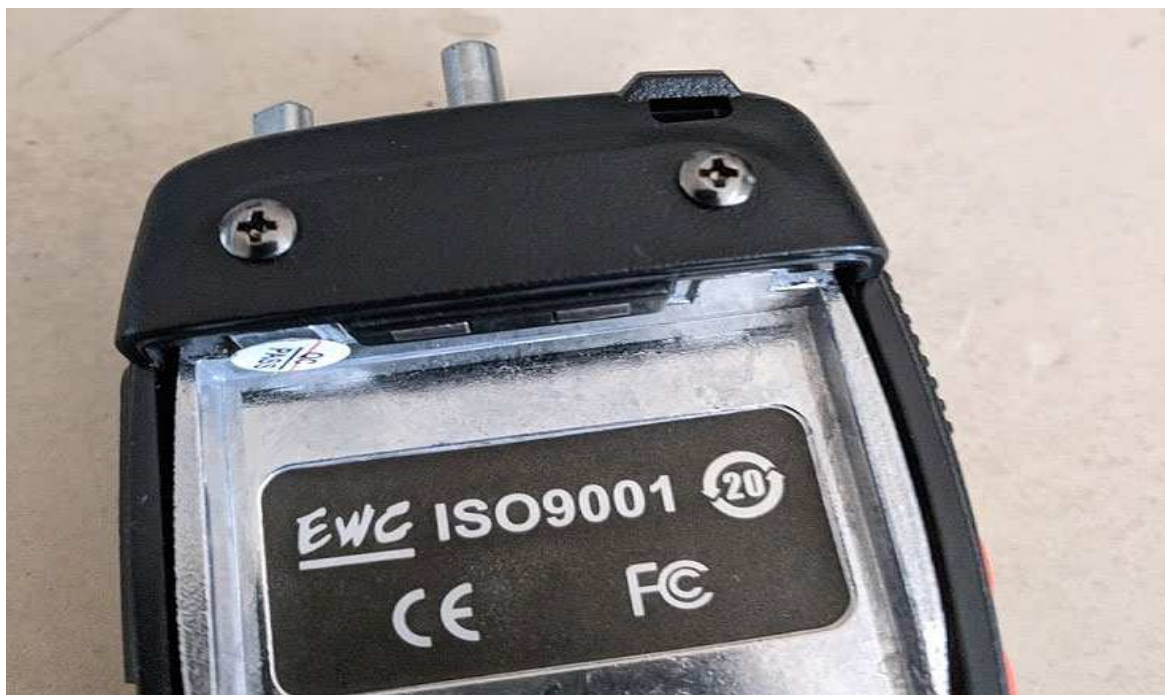
Photo 3. Phillips screws location
