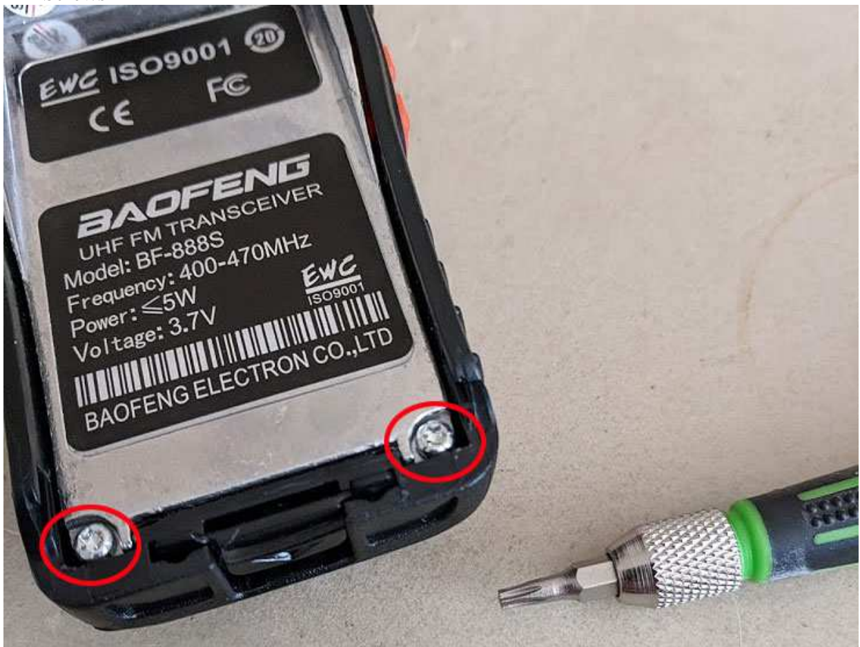
Photo 2. Location of Torx screws
