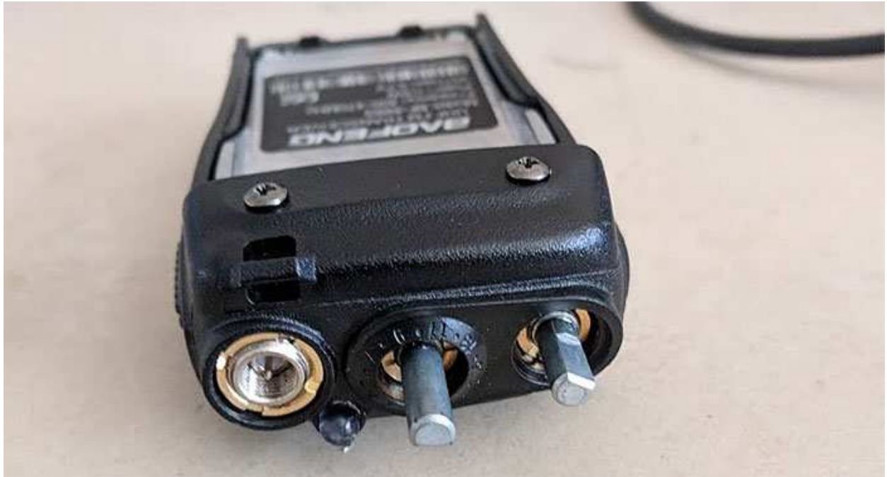
Photo 1. Battery Pack, Knobs and Antenna removed
