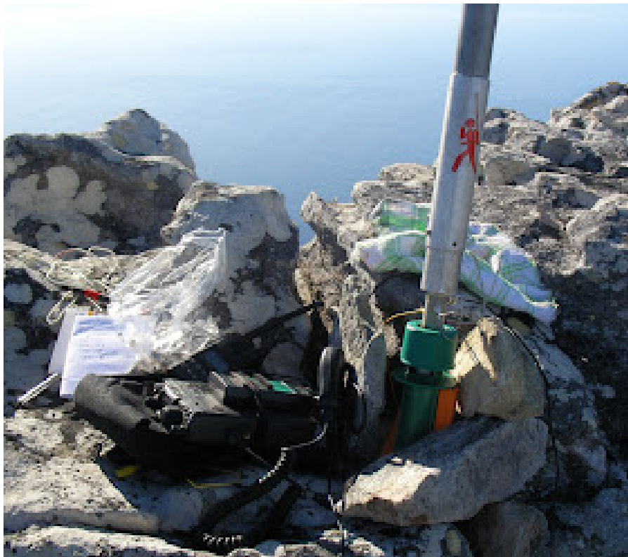
My radio equipment (FT 817 and Elecraft T1 tuner) and base of my telescopic mast / antenna.
