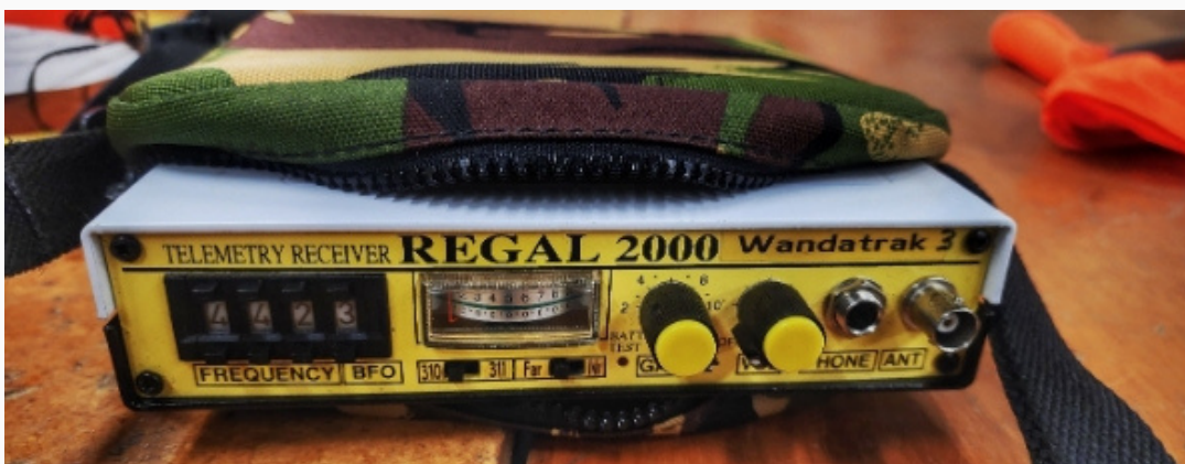
THE REGAL 2000 WANDATRAK 3 – SIMPLISTIC BUT VERY EFFECTIVE – USING RF FREQUENCIES THAT WORK WHERE CELL AND GPS WILL NOT
