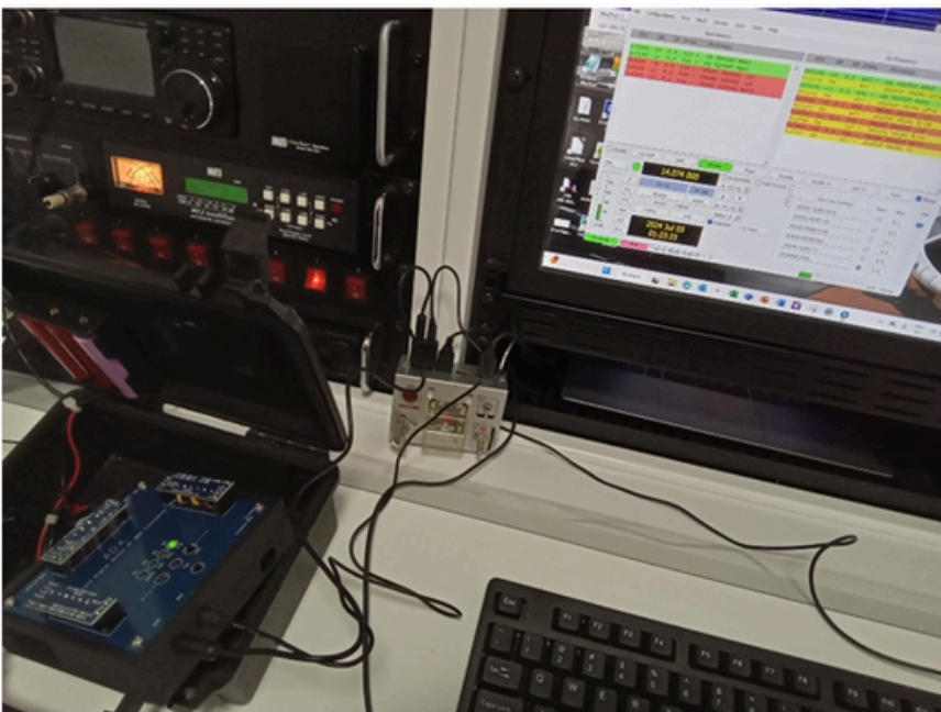
Successful test at home QTH using WSJT-X, three watts into Fiji on 20m. An external USB sound card ( Sabrent ) is used here.
