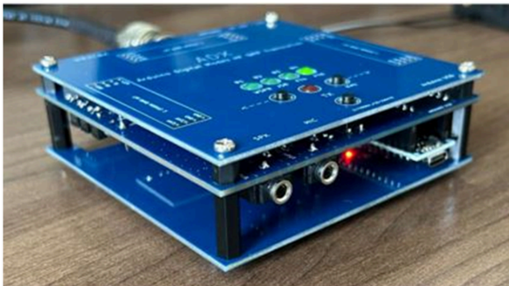
Finished unit with bottom board 'enclosure'; a 3D printed case is also available.
