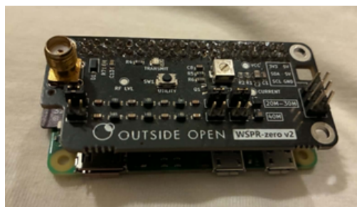
Compact Raspberry Pi-based WSPR transmitter with improved filtering and stability.
