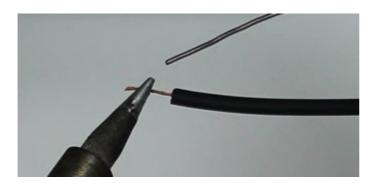
Hold the two tinned wires on top of each other and touch the soldering iron to both wires. This process should melt the solder and coat both wires evenly.
