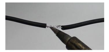
Remove the soldering iron and wait a few seconds to let the soldered connection cool and harden. Use heat shrink to cover the connection.
