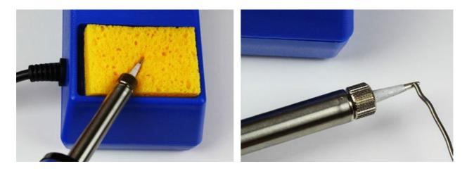
You should tin the tip of your iron before and after each soldering session to extend its life. Eventually, every tip will wear out and will need replacing when it becomes rough or pitted.
