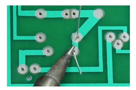
**Step 3: Apply Solder To Joint** – Continue holding the soldering iron on the copper pad and the lead and touch your solder to the joint. **IMPORTANT** – Don't touch the solder directly to the tip of the iron. You want the joint to be hot enough to melt the solder when it's touched. If the joint is too cold, it will form a bad connection.
