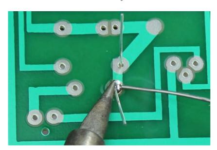
**Step 4: Snip The Leads** – Remove the soldering iron and let the solder cool down naturally. Don't blow on the solder as this will cause a bad joint. Once cool, you can snip the extra wire from leads.
