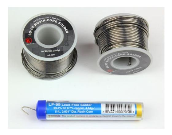
When buying solder, make sure NOT to use acid core solder as this will damage your circuits and components. Acid core solder is sold at home improvement stores and is mainly used for plumbing and metal working.
