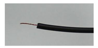
Make sure your soldering iron is fully heated and touch the tip to the end of one of the wires. Hold it on the wire for 3-4 seconds.
