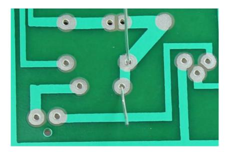
**Step 2: Heat The Joint** – Turn your soldering iron on and if it has an adjustable heat control, set it to 400°C. At this point, touch the tip of the iron to the copper pad and the resistor lead at the same time. You need to hold the soldering iron in place for 3-4 seconds in order to heat the pad and the lead.
